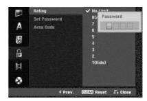
Enter a 4-digit password using the numbered buttons to confirm the personal 4-digit security password.
